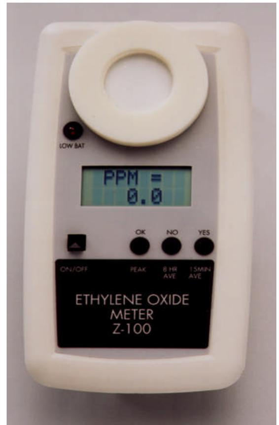
**Z-100 Ethylene Oxide Meter**
